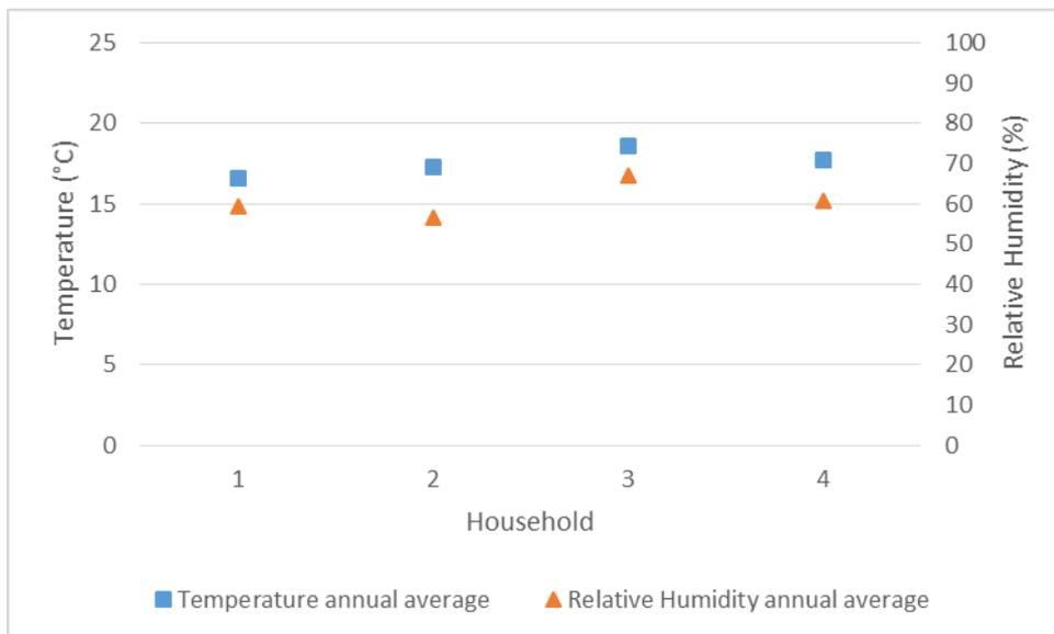
Fig. 18 Recorded internal temperature and relative humidity after ASHP was installed
