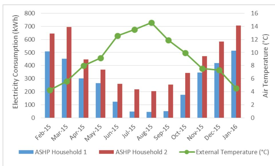
Fig. 8 Monthly total ASHP electricity consumption, and average monthly external air temperature
