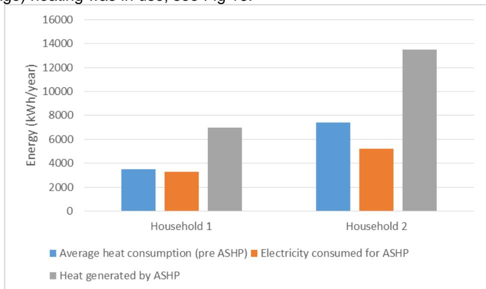
Fig. 16 Comparison of heat consumed before and after installation of ASHP
